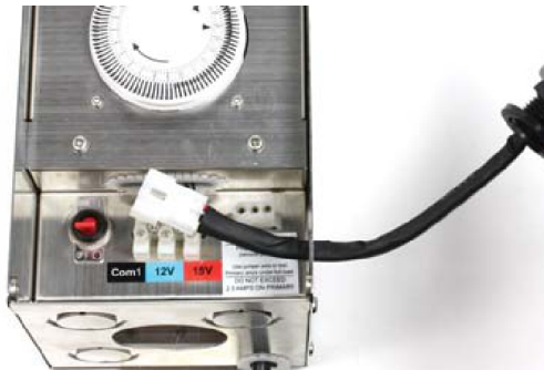
Plug the photo cell into the now empty socket connection.
